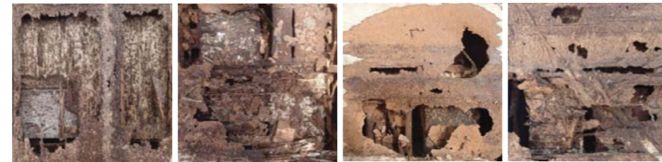
Example of attack by C. acinaciformis termites to bait-wood after 38 weeks' exposure in a Hazard Class H3 field trial.
