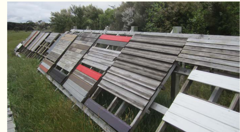
Flat panel test racks, Mangere.
