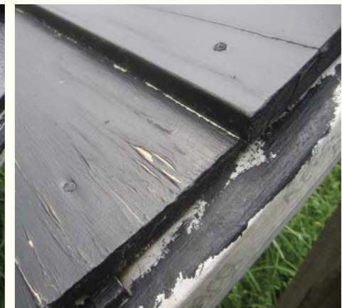
Pressure Treated Clear Grade Radiata Pine, Painted black, 3 years exposure.
