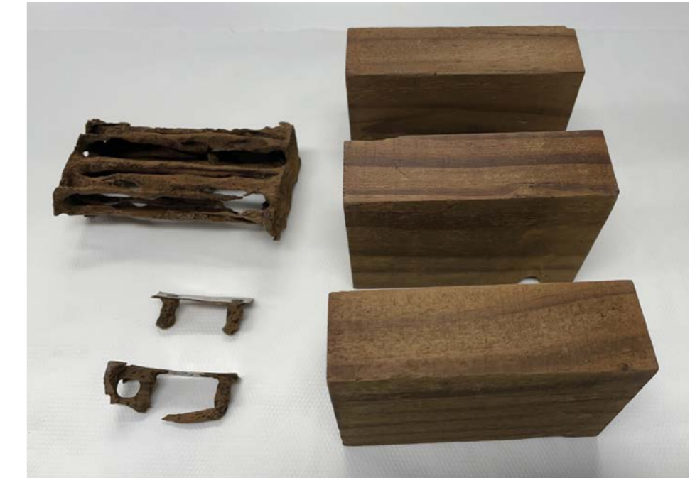
Comparative performance of Imbue Radiata 230°C untreated (left) vs LOSP Azole and permethrin treated (right), when exposed to Coptotermes acinaciformis termites in AWPC H3 field test, Queensland.
